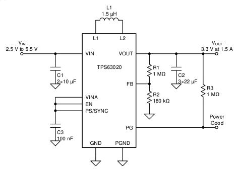
Figure 7. Application Circuit
