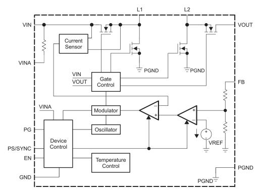
Figure 4. Functional Block Diagram (TPS63021)
