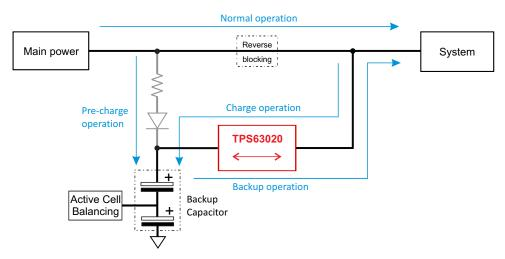
Figure 29. Simplified Block Diagram of a Backup Power System
