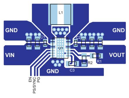
Figure 31. PCB Layout Suggestion
