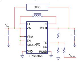
Figure 30. Low-Power TEC Driver Schematic
