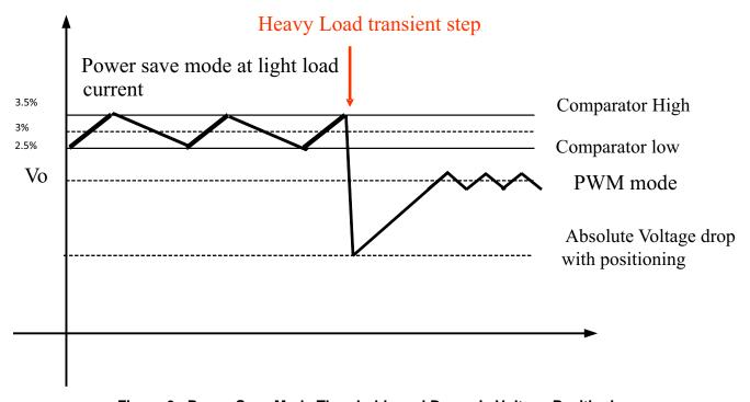
Figure 6. Power Save Mode Thresholds and Dynamic Voltage Positioning
