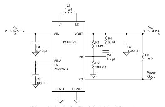
Figure 28. Application Circuit for 2 A Load Current
