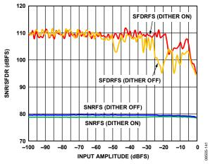
Figure 41. AD9255-125 Single-Tone SNR/SFDR vs. Input Amplitude (A<sub>IN</sub>) with  $f_{\rm IN}$  = 30 MHz With and Without Dither Enabled
