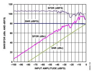
Figure 39. AD9255-125 Single-Tone SNR/SFDR vs. Input Amplitude (A\_{IN}) with  $f_{I\!I\!N}$  = 2.4 MHz
