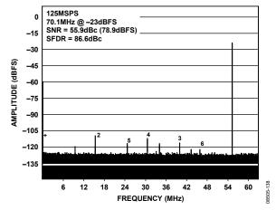
Figure 38. AD9255-125 Single-Tone FFT with  $f_{\rm IN}$  = 70.1 MHz at -23 dBFS with Dither Enabled, 1M Sample
