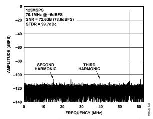
Figure 36. AD9255-125 Single-Tone FFT with  $f_{\rm IN}$  = 70.1 MHz at -6 dBFS with Dither Enabled
