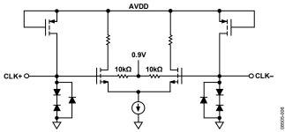
Figure 54. Equivalent Clock Input Circuit
