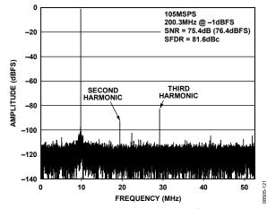
Figure 21. AD9255-105 Single-Tone FFT with  $f_{\rm IN}$  = 200.3 MHz
