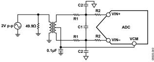
Figure 67. Differential Transformer-Coupled Configuration
