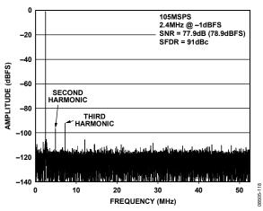
Figure 18. AD9255-105 Single-Tone FFT with  $f_{IN} = 2.4$  MHz
