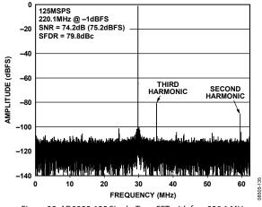
Figure 35. AD9255-125 Single-Tone FFT with  $f_{IN} = 220.1$  MHz
