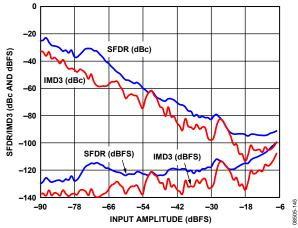
Figure 45. AD9255-125 Two-Tone SFDR/IMD3 vs. Input Amplitude (A<sub>IN</sub>) with  $f_{IN1} = 169.1$  MHz,  $f_{IN2} = 172.1$  MHz,  $f_S = 125$  MSPS
