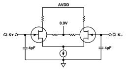
Figure 74. Equivalent Clock Input Circuit
