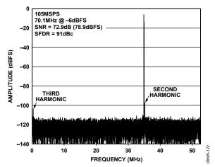
Figure 22. AD9255-105 Single-Tone FFT with f<sub>IN</sub> = 70.1 MHz at −6 dBFS with Dither Enabled
