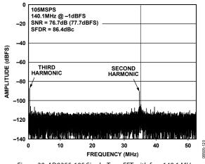
Figure 20. AD9255-105 Single-Tone FFT with  $f_{IN} = 140.1 \text{ MHz}$
