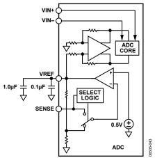
Figure 70. Internal Reference Configuration
