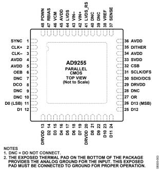
*Figure 4. LFCSP Parallel CMOS Pin Configuration (Top View)*
