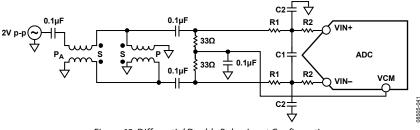
Figure 68. Differential Double Balun Input Configuration
