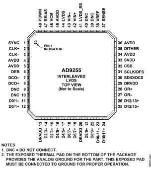
Figure 5. LFCSP Interleaved Parallel LVDS Pin Configuration (Top View)
