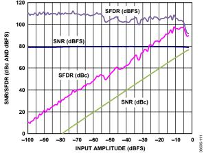
Figure 11. AD9255-80 Single-Tone SNR/SFDR vs. Input Amplitude (A<sub>IN</sub>) with  $f_{IN} = 98.12 \text{ MHz}$
