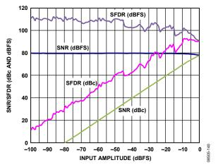
Figure 40. AD9255-125 Single-Tone SNR/SFDR vs. Input Amplitude (A\_{IN}) with  $f_{\rm IN}=98.12~\rm MHz$
