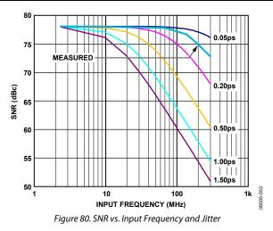
Treat the clock input as an analog signal in cases in which aperture jitter may affect the dynamic range of the AD9255. To avoid modulating the clock signal with digital noise, separate power supplies for clock drivers from the ADC output driver supplies. Low jitter, crystal controlled oscillators make the best clock sources. If the clock is generated from another type of source (by gating, dividing, or another method), the output clock should be retimed by the original clock at the last step.
