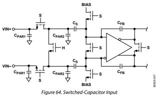
For best dynamic performance, the source impedances driving VIN+ and VIN- should be matched, and the inputs should be differentially balanced.
