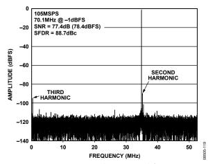
Figure 19. AD9255-105 Single-Tone FFT with  $f_{IN} = 70.1 \text{ MHz}$
