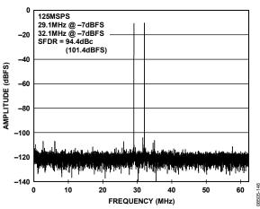
Figure 46. AD9255-125 Two-Tone FFT with  $f_{IN1} = 29.1$  MHz and  $f_{IN2} = 32.1$  MHz
