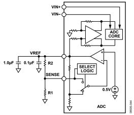
Figure 71. Programmable Reference Configuration
