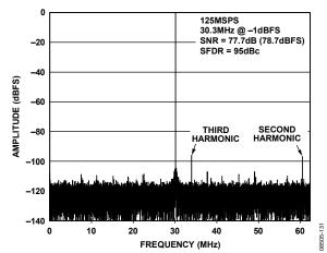
Figure 31. AD9255-125 Single-Tone FFT with  $f_{IN}$  = 30.3 MHz
