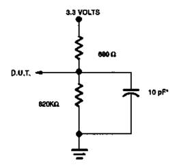
\* INCLUDING SCOPE AND JIG CAPACITANCE
