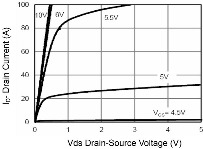
Figure 1 Output Characteristics
