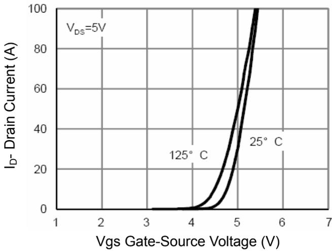
Figure 2 Transfer Characteristics
