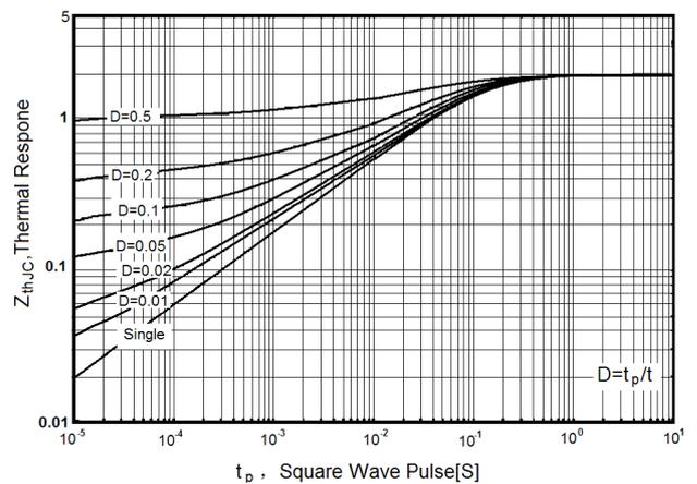
Figure13. Transient Thermal Impedance for TO-220F
