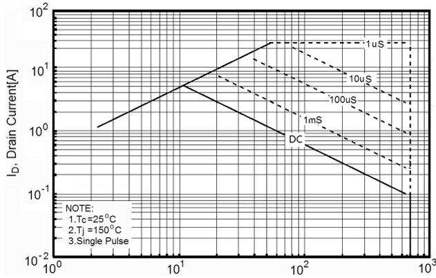
Figure2. Safe operating area for TO-220F
