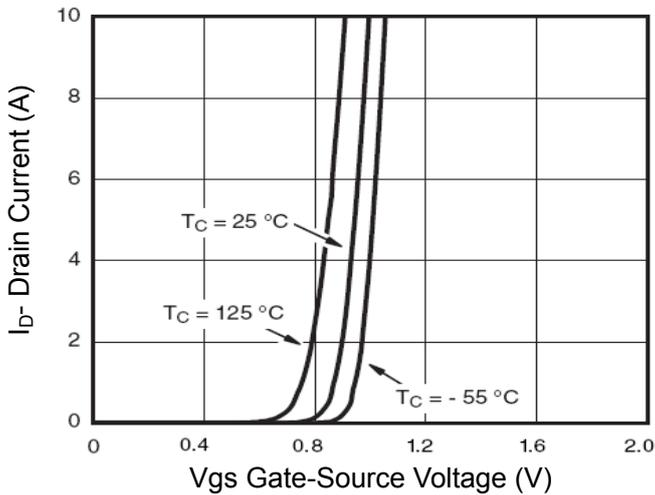
Figure 2 Transfer Characteristics
