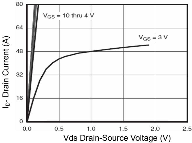
Figure 1 Output Characteristics
