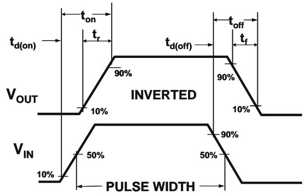
Figure 2: Switching Waveforms
