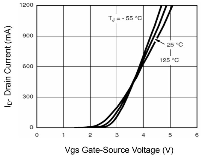
Figure 4 Transfer Characteristics
