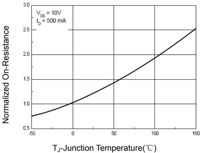
**Figure 9 Drain-Source On-Resistance**
