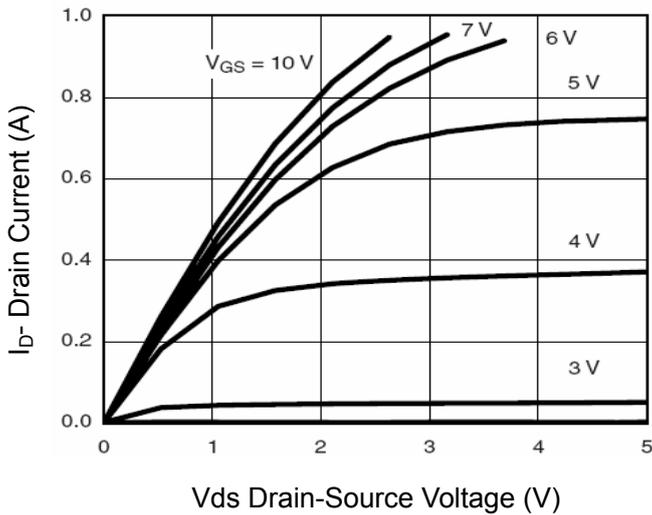
Figure 3 Output Characteristics
