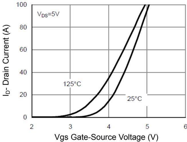
**Figure 2 Transfer Characteristics**
