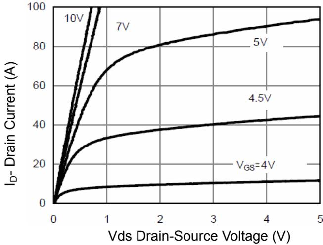
**Figure 1 Output Characteristics**
