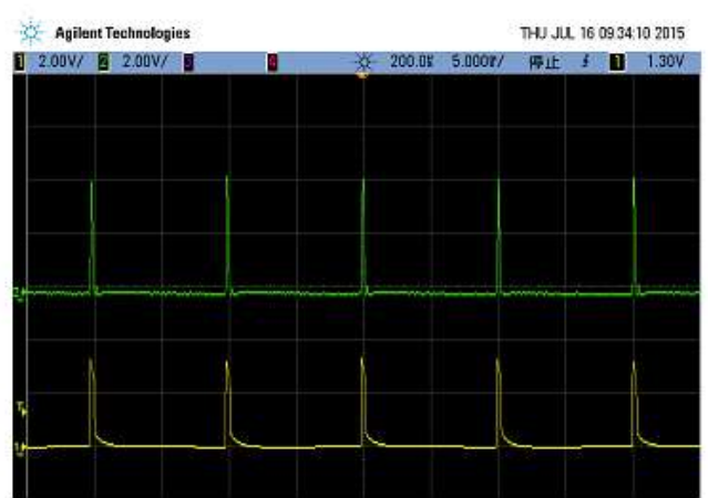
Figure 2 Performance of dust detection by infrared pulse stimulation
