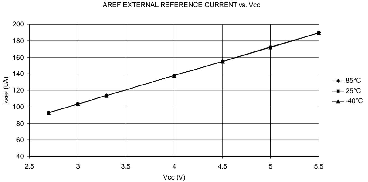
**Figure 28-35.** Analog Comparator Current vs. Operating Voltage
