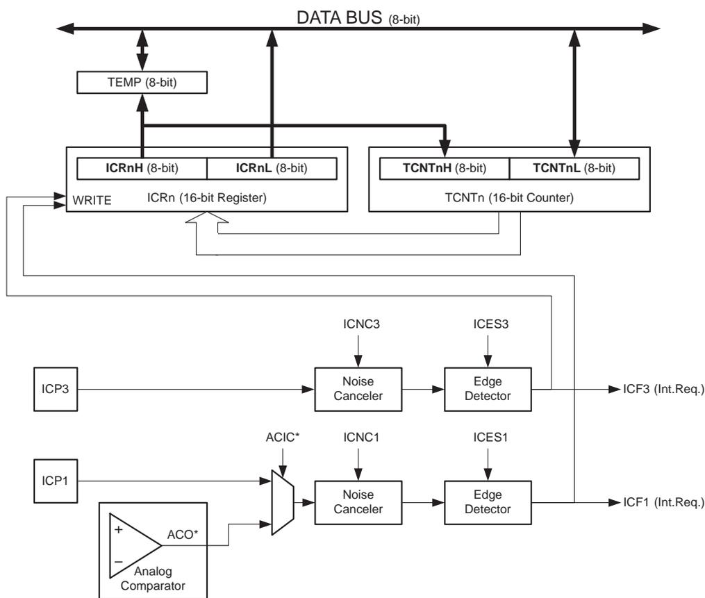
Note: The Analog Comparator Output (ACO) can only trigger the Timer/Counter1 IC Unit– not Timer/Counter3.
