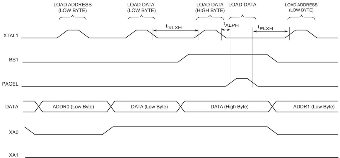
Note: 1. The timing requirements shown in Figure 26-10 (i.e.,  $t_{DVXH}$ ,  $t_{XHXL}$ , and  $t_{XLDX}$ ) also apply to loading operation.
