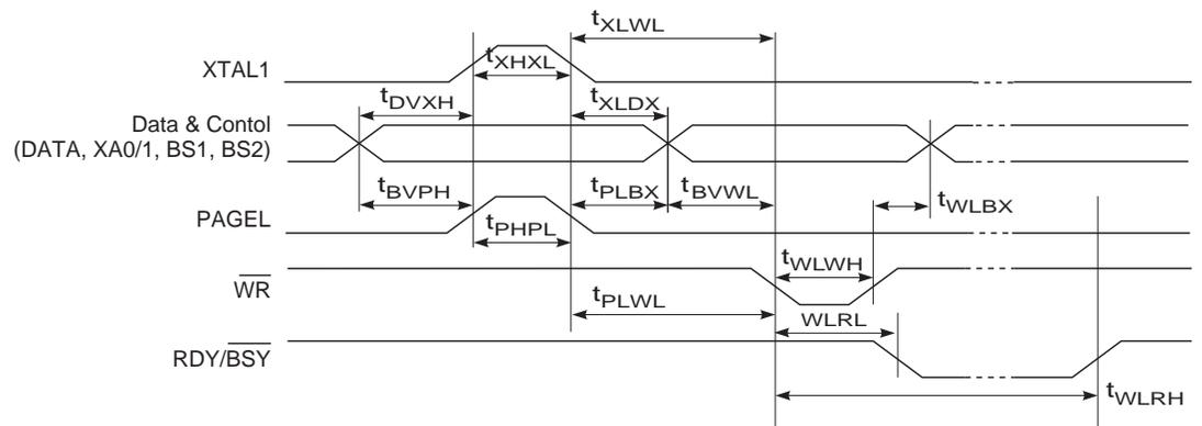
**Figure 26-11.** Parallel Programming Timing, Loading Sequence with Timing Requirements<sup>(1)</sup>
