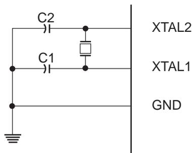
The Oscillator can operate in three different modes, each optimized for a specific frequency range. The operating mode is selected by the fuses CKSEL3..1 as shown in [Table 5-3](#).
