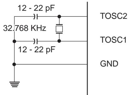
A external clock can also be used using TOSC1 as input. Setting AS2 and EXCLK enables this configuration.
