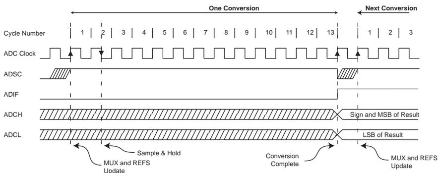
**Figure 21-6.** ADC Timing Diagram, Auto Triggered Conversion
