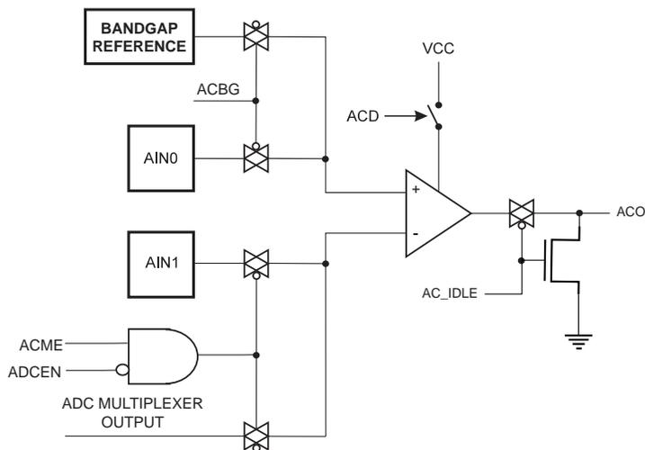
Figure 23-9. General Boundary-scan cell Used for Signals for Comparator and ADC
