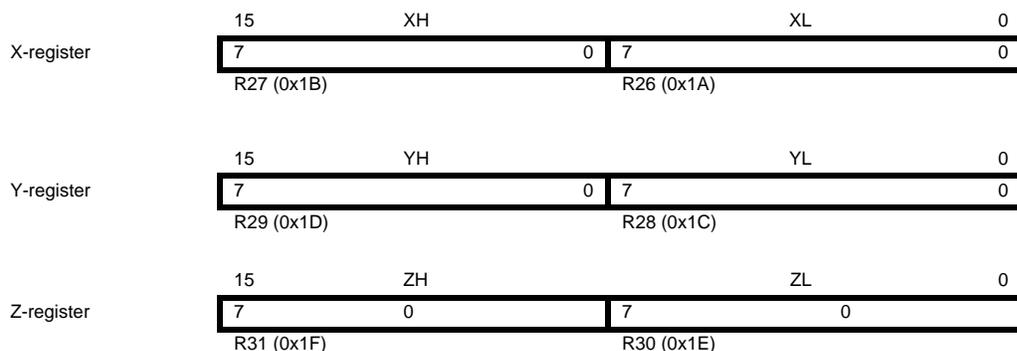
In the different addressing modes these address registers have functions as fixed displacement, automatic increment, and automatic decrement (see the instruction set reference for details).
