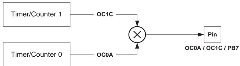
When the modulator is enabled, the two output compare channels are modulated together as shown in the block diagram (Figure 15-1).
