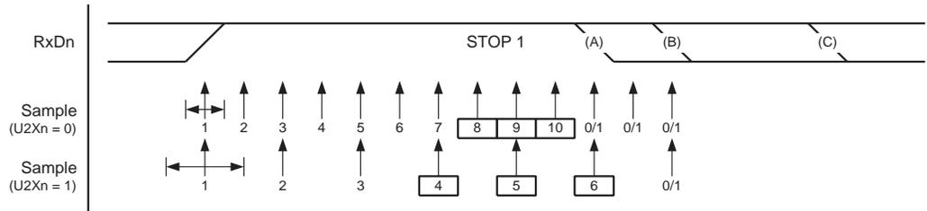
The same majority voting is done to the stop bit as done for the other bits in the frame. If the stop bit is registered to have a logic 0 value, the Frame Error (FEn) flag will be set.
