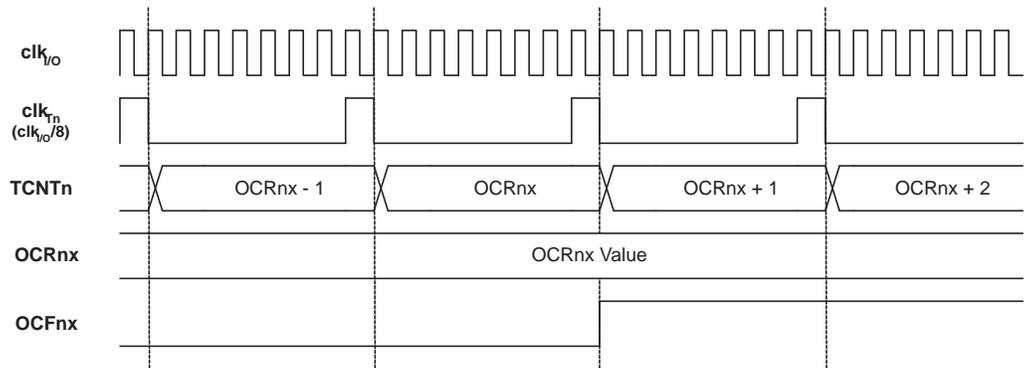
Figure 14-12 shows the setting of OCF2A and the clearing of TCNT2 in CTC mode.
