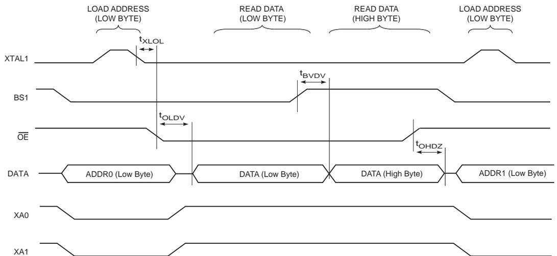
Note: 1. The timing requirements shown in Figure 26-10 (i.e.,  $t_{DVXH}$ ,  $t_{XHXL}$ , and  $t_{XLDX}$ ) also apply to reading operation.
