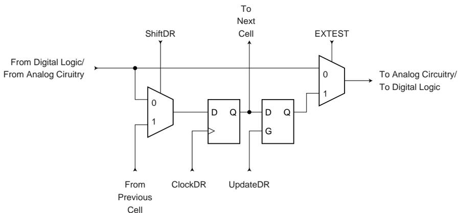
Table 23-6. Boundary-scan Signals for the Analog Comparator
