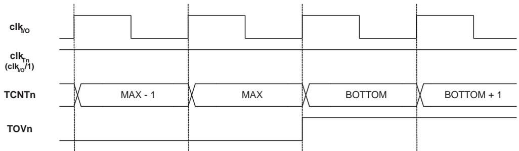
Figure 14-10 shows the same timing data, but with the prescaler enabled.
