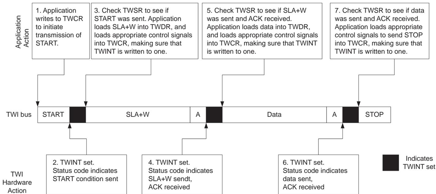
1. The first step in a TWI transmission is to transmit a START condition. This is done by writing a specific value into TWCR, instructing the TWI hardware to transmit a START condition. Which value to write is described later on. However, it is important that the TWINT bit is set in the value written. Writing a one to TWINT clears the flag. The TWI will not start any operation as long as the TWINT bit in TWCR is set. Immediately after
