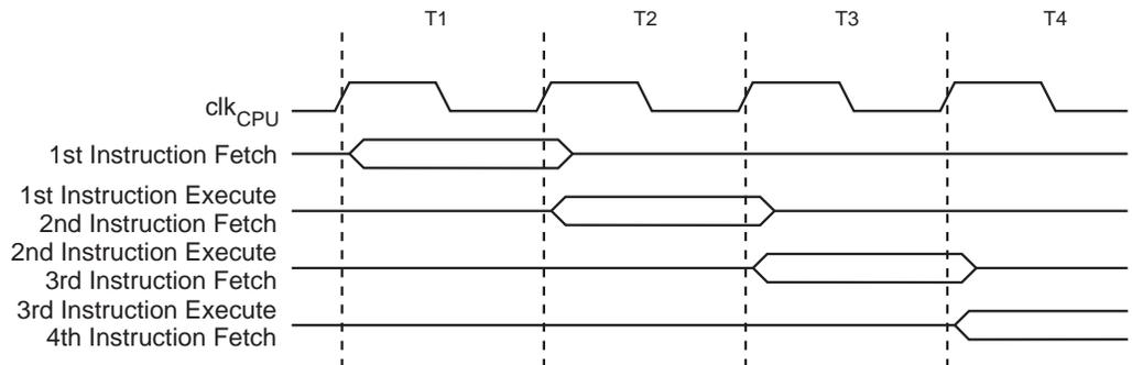
Figure 3-6 shows the internal timing concept for the Register File. In a single clock cycle an ALU operation using two register operands is executed, and the result is stored back to the destination register.
