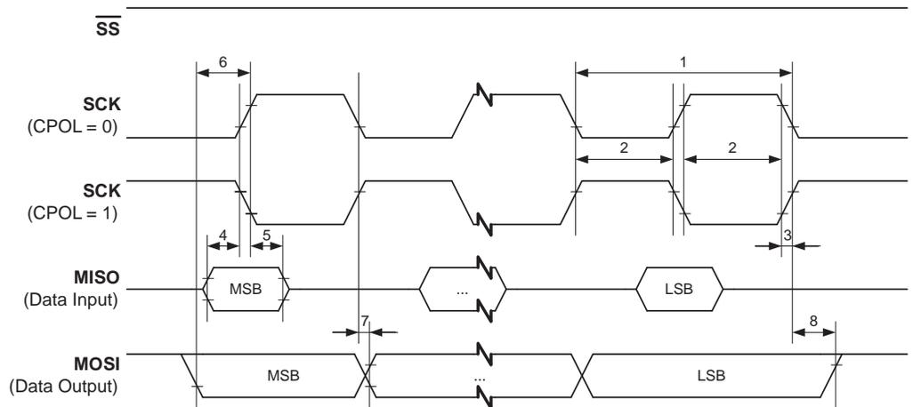
**Figure 26-5.** SPI Interface Timing Requirements (Slave Mode)
