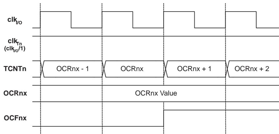
[Figure 13-11](#) shows the same timing data, but with the prescaler enabled.
