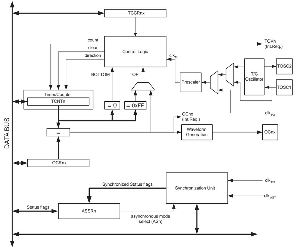
The Timer/Counter (TCNT2) and Output Compare Register (OCR2A) are 8-bit registers. Interrupt request (shortened as Int.Req.) signals are all visible in the Timer Interrupt Flag Register (TIFR2). All interrupts are individually masked with the Timer Interrupt Mask Register (TIMSK2). TIFR2 and TIMSK2 are not shown in the figure.
