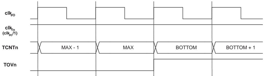
[Figure 12-9](#) shows the same timing data, but with the prescaler enabled.
