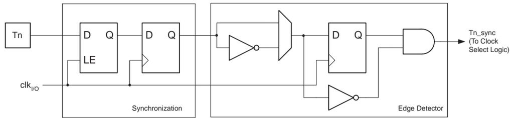
The synchronization and edge detector logic introduces a delay of 2.5 to 3.5 system clock cycles from an edge has been applied to the T3/T1/T0 pin to the counter is updated.
