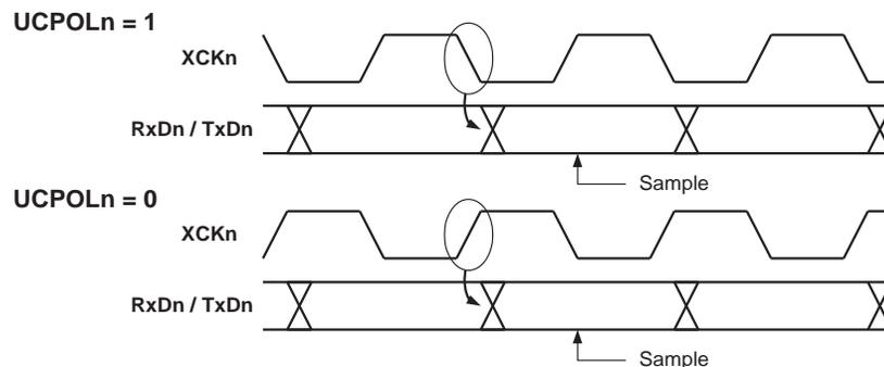
The UCPOLn bit UCRSnC selects which XCKn clock edge is used for data sampling and which is used for data change. As Figure 17-3 shows, when UCPOLn is zero the data will be changed at rising XCKn edge and sampled at falling XCKn edge. If UCPOLn is set, the data will be changed at falling XCKn edge and sampled at rising XCKn edge.
