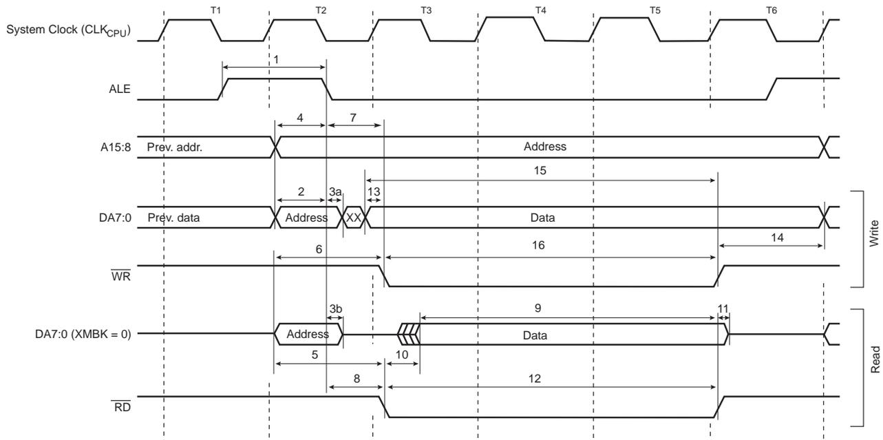
**Figure 26-9.** External Memory Timing (SRWn1 = 1, SRWn0 = 1)<sup>(1)</sup>
