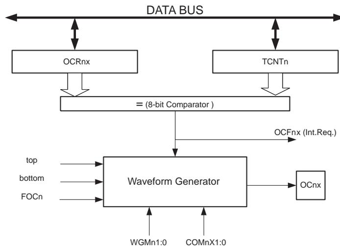
The OCR2A Register is double buffered when using any of the Pulse Width Modulation (PWM) modes. For the Normal and Clear Timer on Compare (CTC) modes of operation, the double buffering is disabled. The double buffering synchronizes the update of the OCR2A Compare
