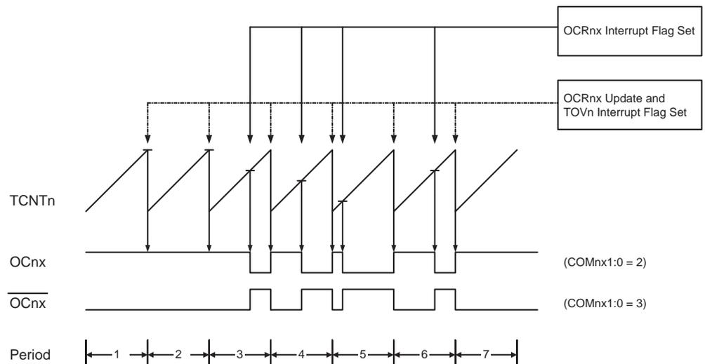
The Timer/Counter Overflow Flag (TOV2) is set each time the counter reaches MAX. If the interrupt is enabled, the interrupt handler routine can be used for updating the compare value.
