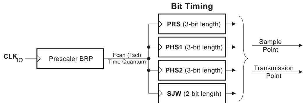
**Figure 19-8.** General Structure of a Bit Period
