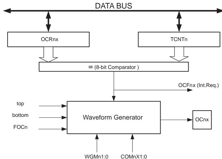
The OCR0A Register is double buffered when using any of the Pulse Width Modulation (PWM) modes. For the normal and Clear Timer on Compare (CTC) modes of operation, the double buffering is disabled. The double buffering synchronizes the update of the OCR0A Compare Register to either top or bottom of the counting sequence. The synchronization prevents the occurrence of odd-length, non-symmetrical PWM pulses, thereby making the output glitch-free.
