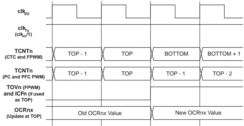
Figure 13-13 shows the same timing data, but with the prescaler enabled.
