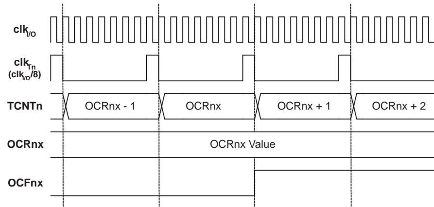
[Figure 13-12](#) shows the count sequence close to TOP in various modes. When using phase and frequency correct PWM mode the OCRnx Register is updated at BOTTOM. The timing diagrams will be the same, but TOP should be replaced by BOTTOM, TOP-1 by BOTTOM+1 and so on. The same renaming applies for modes that set the TOVn flag at BOTTOM.
