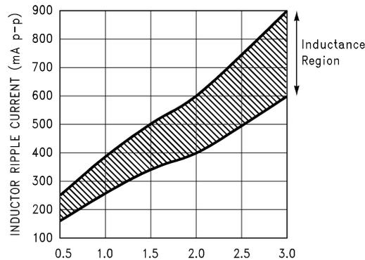
**Figure 30. Peak-to-Peak Inductor Ripple Current vs Load Current**
