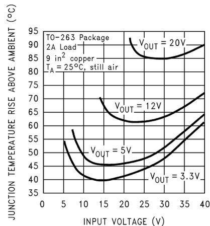
Circuit Data for Temperature Rise Curve
