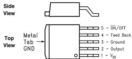
**Figure 2. 5-Lead DDPAK/TO-263 (S) Package**
