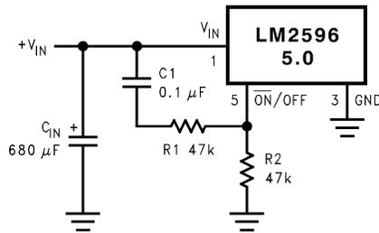
Figure 33. Delayed Startup
