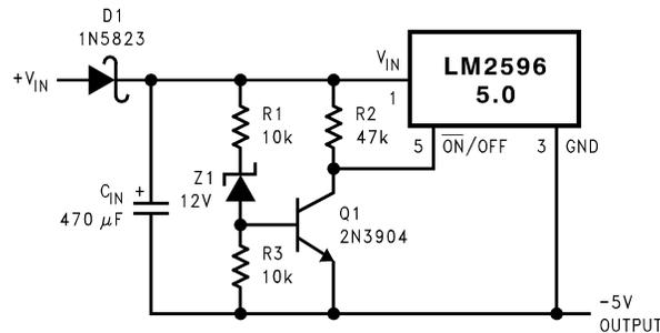
This circuit has an ON/OFF threshold of approximately 13V.
