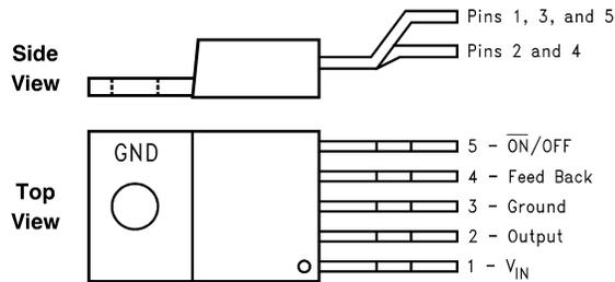
**Figure 1. 5-Lead Bent and Staggered Leads, Through Hole TO-220 (T) Package**
