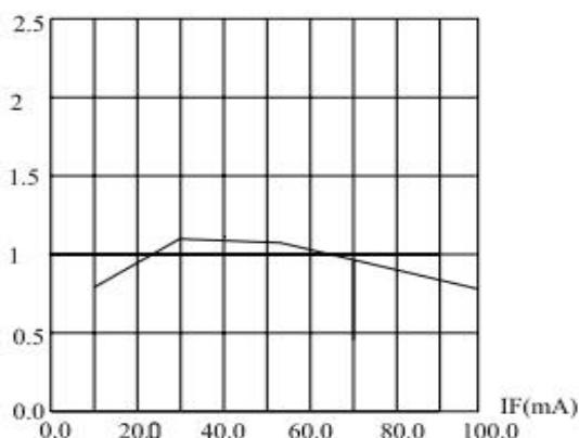
FIG.3 RELATIVE LUMINOUS INTENSITY VS.
