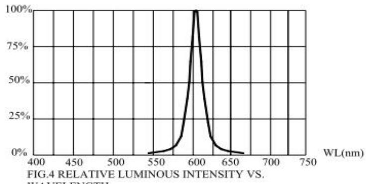
FIG.4 RELATIVE LUMINOUS INTENSITY VS.
