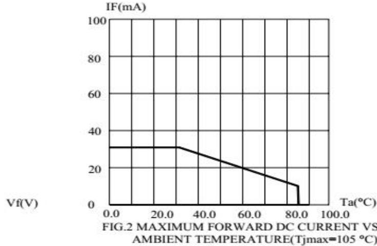
FIG.2 MAXIMUM FORWARD DC CURRENT VS.
