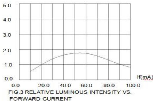
FIG.3 RELATIVE LUMINOUS INTENSITY VS.
