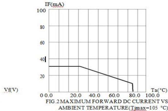
FIG.2 MAXIMUM FORWARD DC CURRENT VS.
