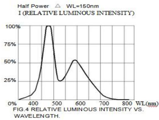
FIG.4 RELATIVE LUMINOUS INTENSITY VS.
