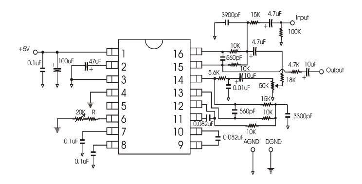
Note: External Resistor having a value of 10 K Ohms to 50 K Ohms may be used. The recommended Resistor Value (R) is 10 K Ohms. When the value of the Resistor (R) increases, the range of the Delay Time also increases.
