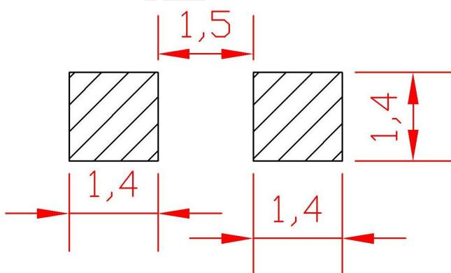
建议焊盘尺寸 (Recommended pad size)
