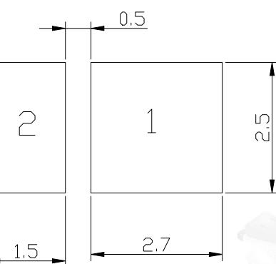
推荐焊盘式样(Recommended Soldering Patter)
