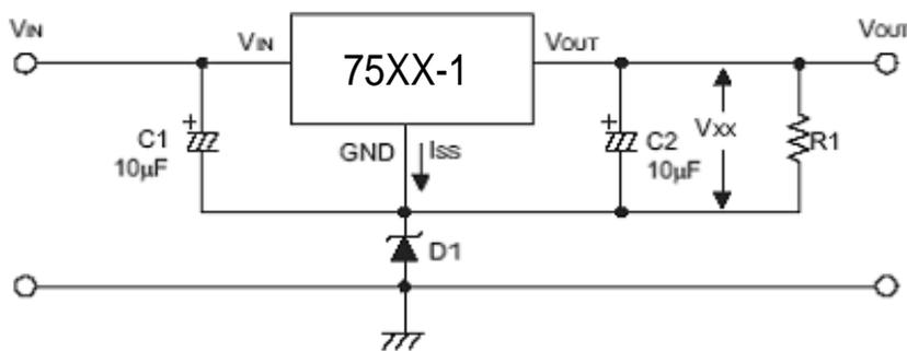
$$V_{OUT} = V_{XX} + VD1$$
