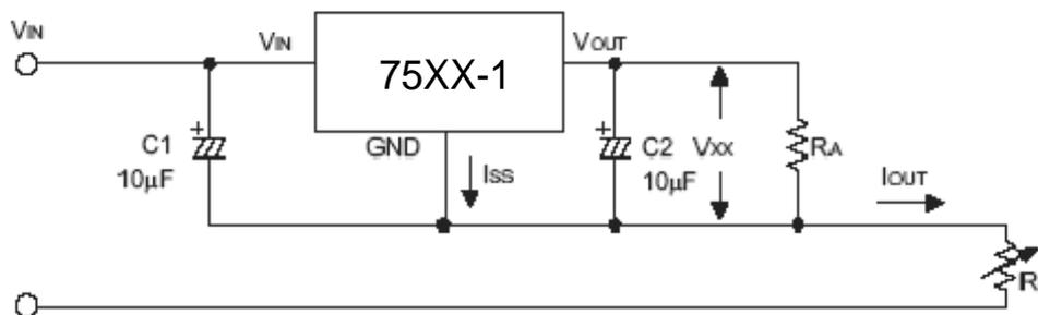
$$I_{OUT} = V_{XX}/R_X + I_{SS}$$
