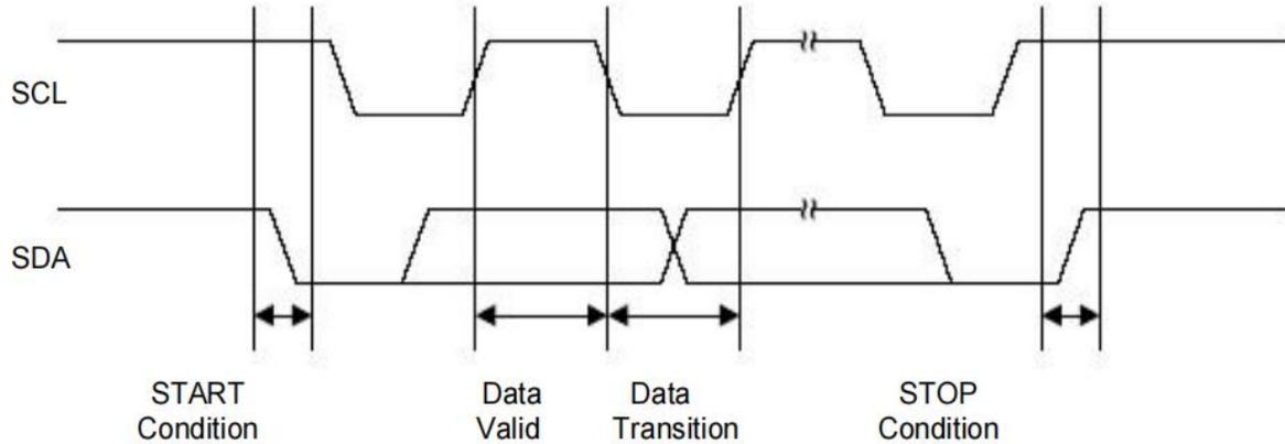
Figure1: Timing diagram for START and STOP conditions
