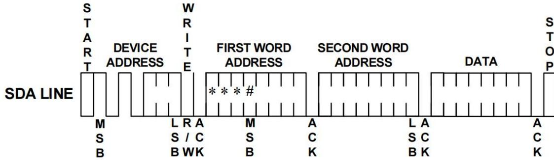
Figure 3: Byte Write
