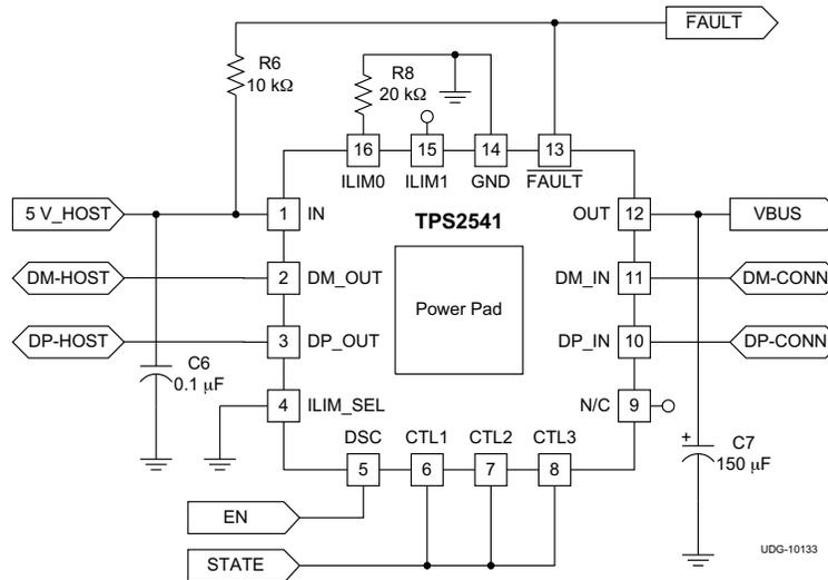
图 44. TPS2541 Application Using Single STATE Control Signal
