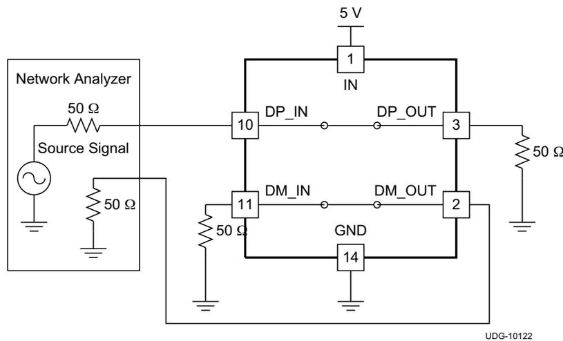
图 37. ON State Cross Channel Isolation ( $X_{TALK}$ )
