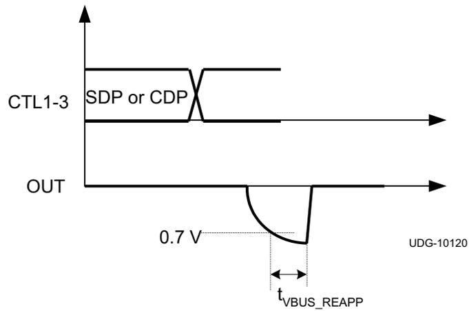
图 33. OUT Discharge During CTLx Lines Change
