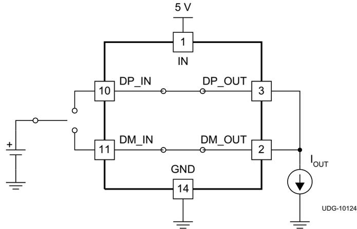
图 40. On Resistance DP/DM High-Speed Switch ( $R_{HS\_ON}$ )
