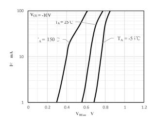
Fig 3 V<sub>BE(sat)</sub> vs. Ic
