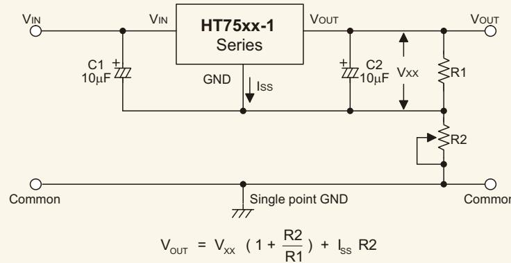
Circuit for Increasing Output Voltage
