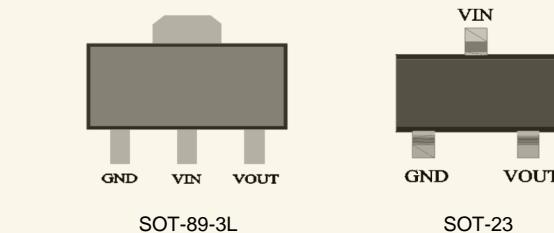
2.1V to 12.0V. CMOS technology ensures low voltage drop and low quiescent current.
