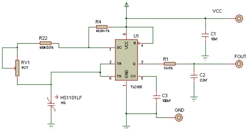
Note: R22=499kΩ / R4=49.9kΩ / R1=1 kΩ / RV1=50 kΩ potentiometer / C1=10nF / C2=2.2nF / C3=100nF
