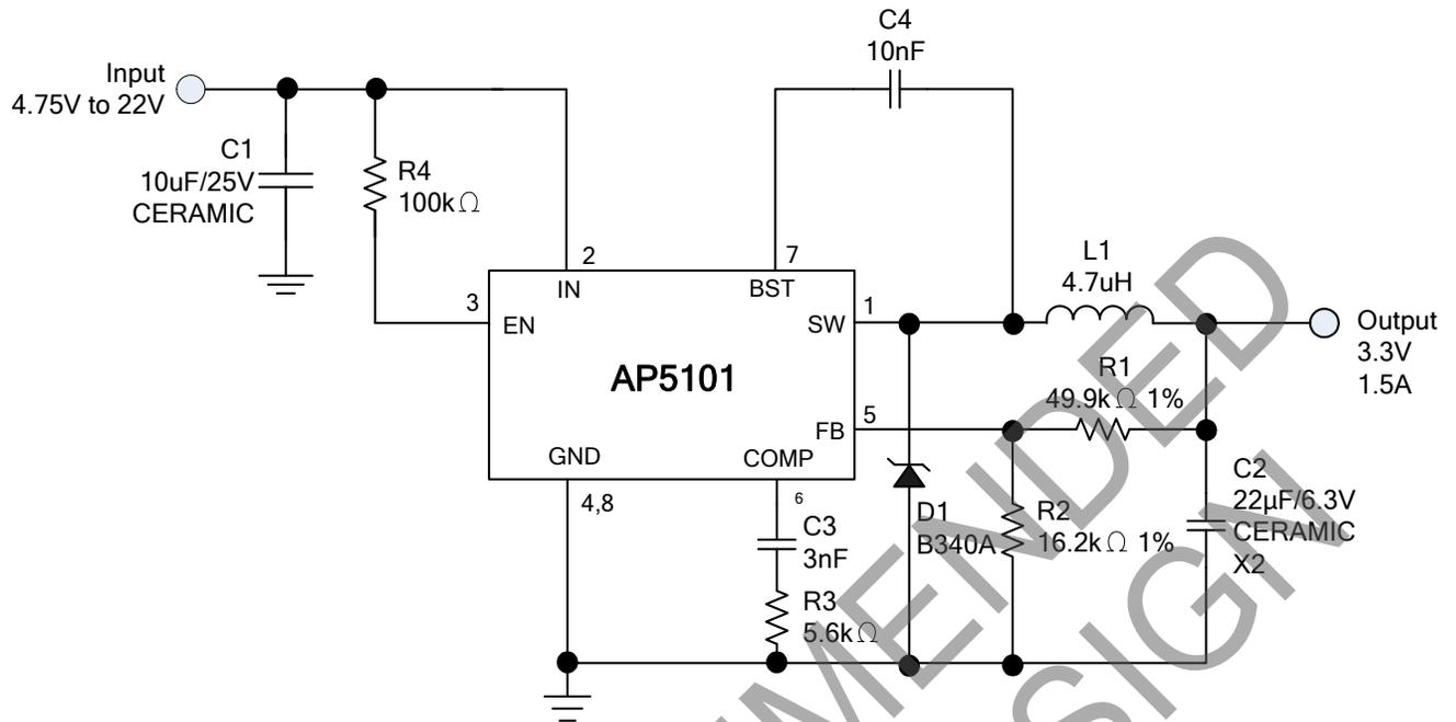
Figure 2. 1.4MHz, 3.3V Output at 1.5A Step-Down Converter
